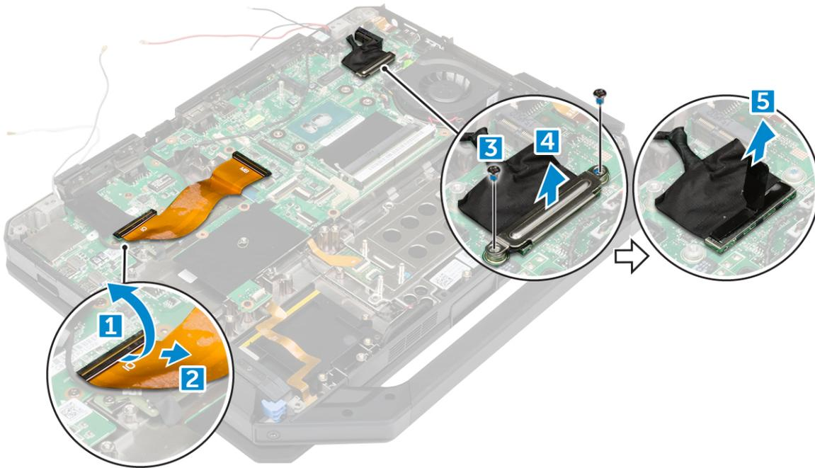
4. Peel the adhesive tape [1] [3] and disconnect the display cables from the connectors [2] [4].
