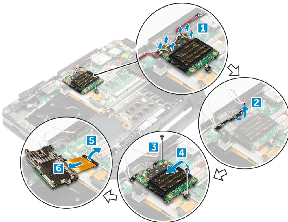
4. Lift and remove the docking board from the computer chassis.
