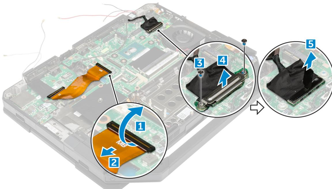
6. Peel the adhesive tape [1] and disconnect the following cables:
