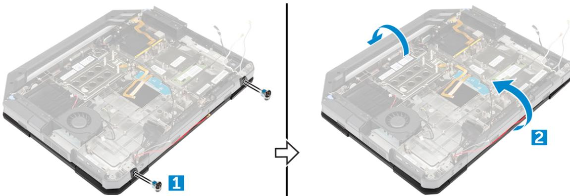
6. Open the display and lift the display assembly away from the computer.
