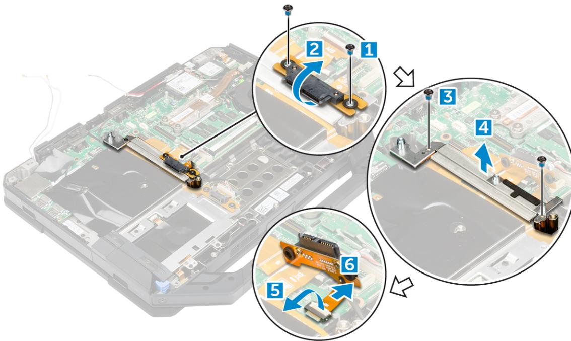
4. Lift the optical drive connector away from the computer.
