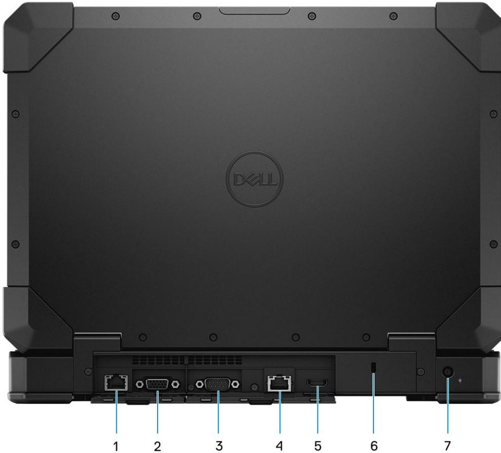
1. Ethernet Port (Optional Rear configurable I/O)
